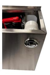
Fit the dual flush push button to the hole in the front of the cistern enclosure. The chrome bezel unscrews from the front and the button is inserted from behind. The large plastic collar then tightens up from behind. Fit the two air tubes from the syphon to the rear of the push button. Instructions are included in the plastic concealed cistern.
